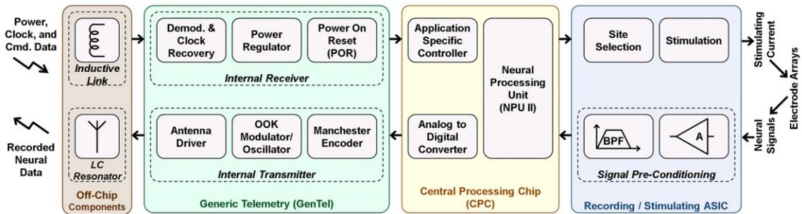
Fig. A.22: Block diagram of the functional organization for the implantable system.
