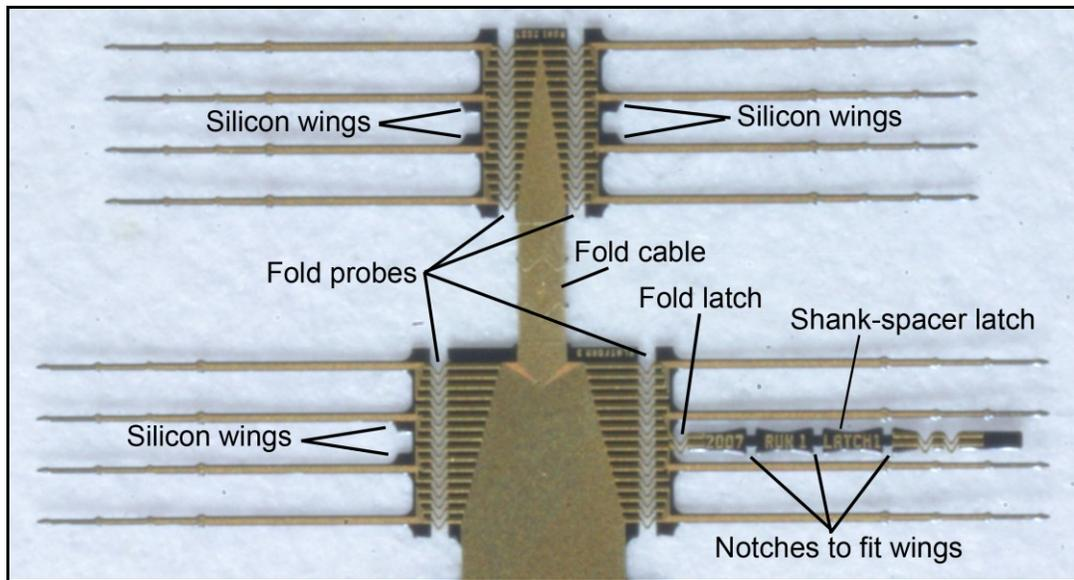
Fig. 5.14: Labeled photograph of the shank-spacer latch design.
