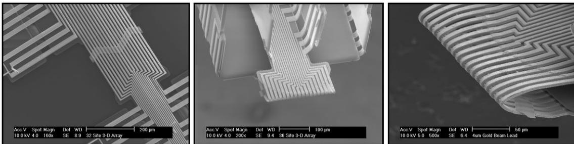
Fig. 5.26: SEM views showing the leads for the platform connector cable.
