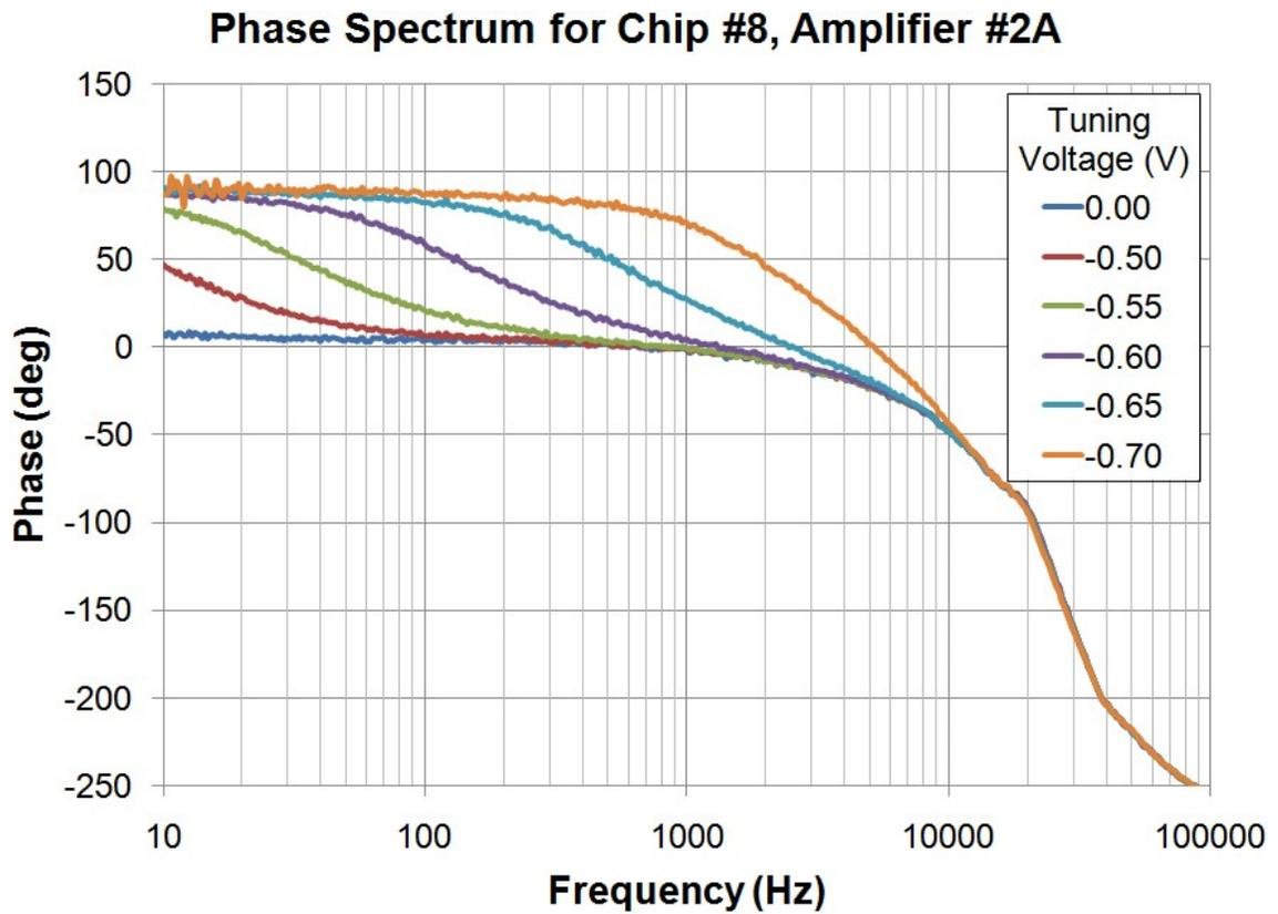
Fig. 4.24: Measured frequency response for chip #8, amplifier #2A.
