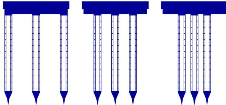
Fig. 2.25: Drawings of the multi-shank probes for the 3-D parallel probe arrays. Shank width is 300 $\mu\text{m}$  and spacing (gap) is 800, 400, and 200 $\mu\text{m}$  (left to right). Solid shank versions were also made.
