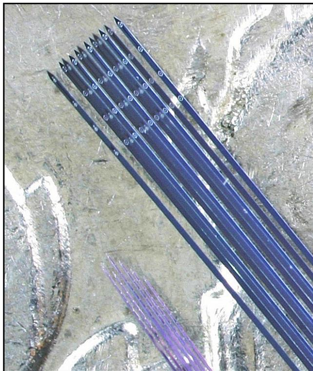
Fig. 6.24: Close-up photograph of VCN-DCN array shanks.
