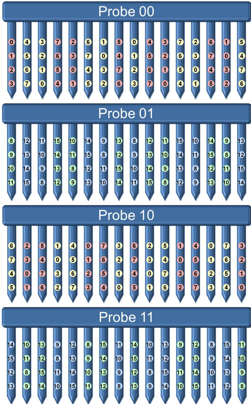
Fig. A.31: Connections between the 32 amplifiers and the electrode sites. The colors indicate one of the two amplifiers within the numbered R/S Unit: red and green signify amplifier A whereas yellow and blue signify amplifier B.
