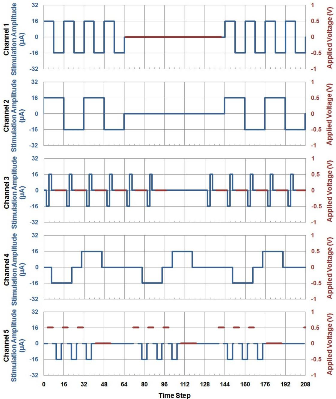
Fig. A.10: Waveforms for Example 2 (1 Time Step =  $13.5\mu\text{s}$  for a 2MHz clock).
