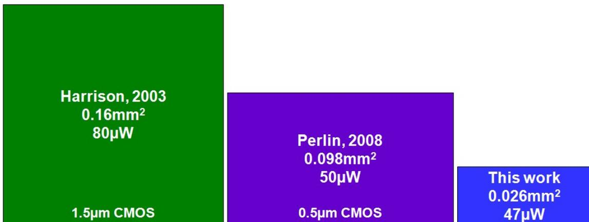
Fig. 4.21: Comparison of per channel size and measured power of neural recording amplifiers [59, 108].
