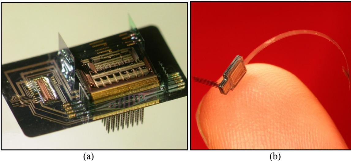
Fig. 1.6: Photos of two low profile 3-D electrode arrays in which (a) the integrated circuit portion of the probe back-ends fold down parallel to the platform [63] and (b) the 500 $\mu$ m thick block platform holds probes and a hybrid chip [59].
