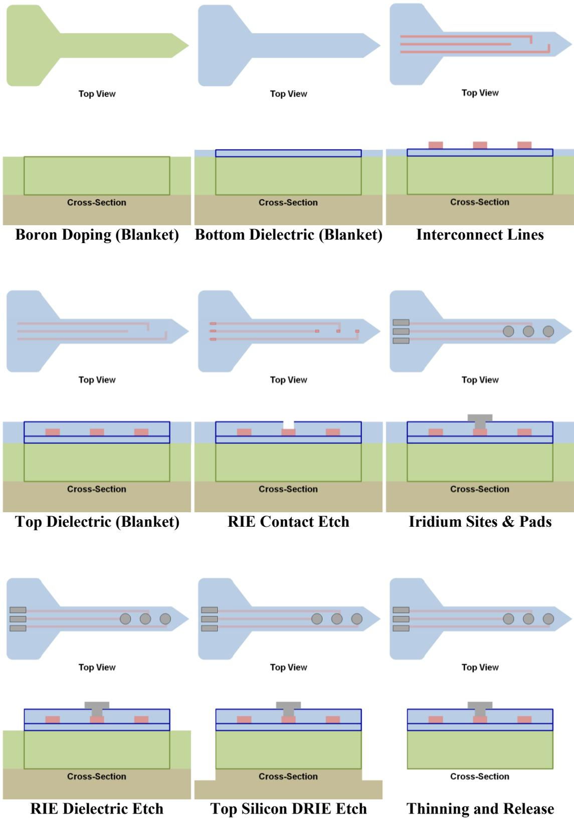
Fig. 3.1: Drawings of the general fabrication steps.
