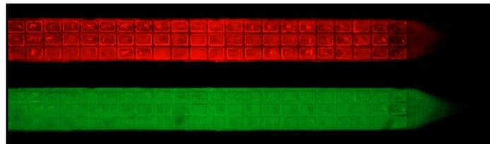
Fig. 2.21: Fluorescent images of coated lattice probes with tethered HPMA polymer functionalized with TexasRed labeled TT (top) and after further functionalization with FITC labeled NH<sub>2</sub> (bottom) [84].
