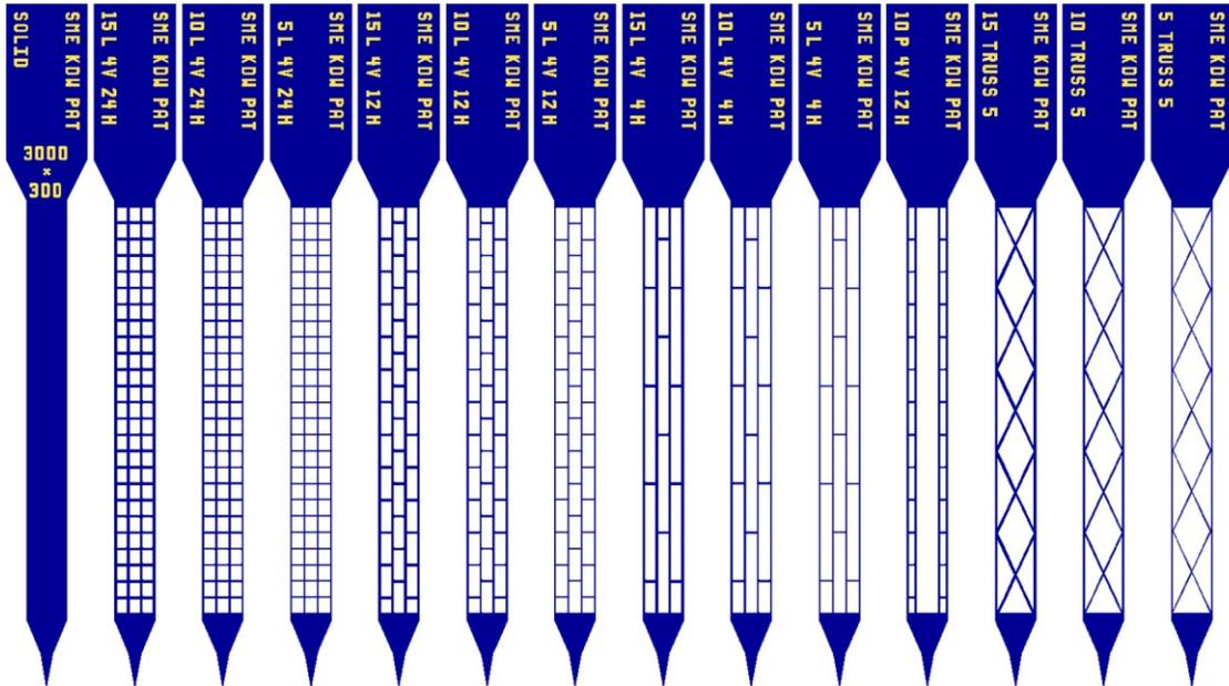
Fig. 2.2: Layout of solid and lattice probe designs (solid, block, brick, picket, and truss) using the standard back-end for the tethered setup. Probes have rib layout widths of 15, 10, and  $5\mu\text{m}$ .
