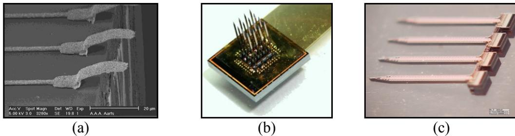
Fig. 1.4: Work done under the NeuroProbe project (a) gold beam-lead clips, (b) a 3-D array prototype, and (c) one probe with integrated circuitry [54, 55].
