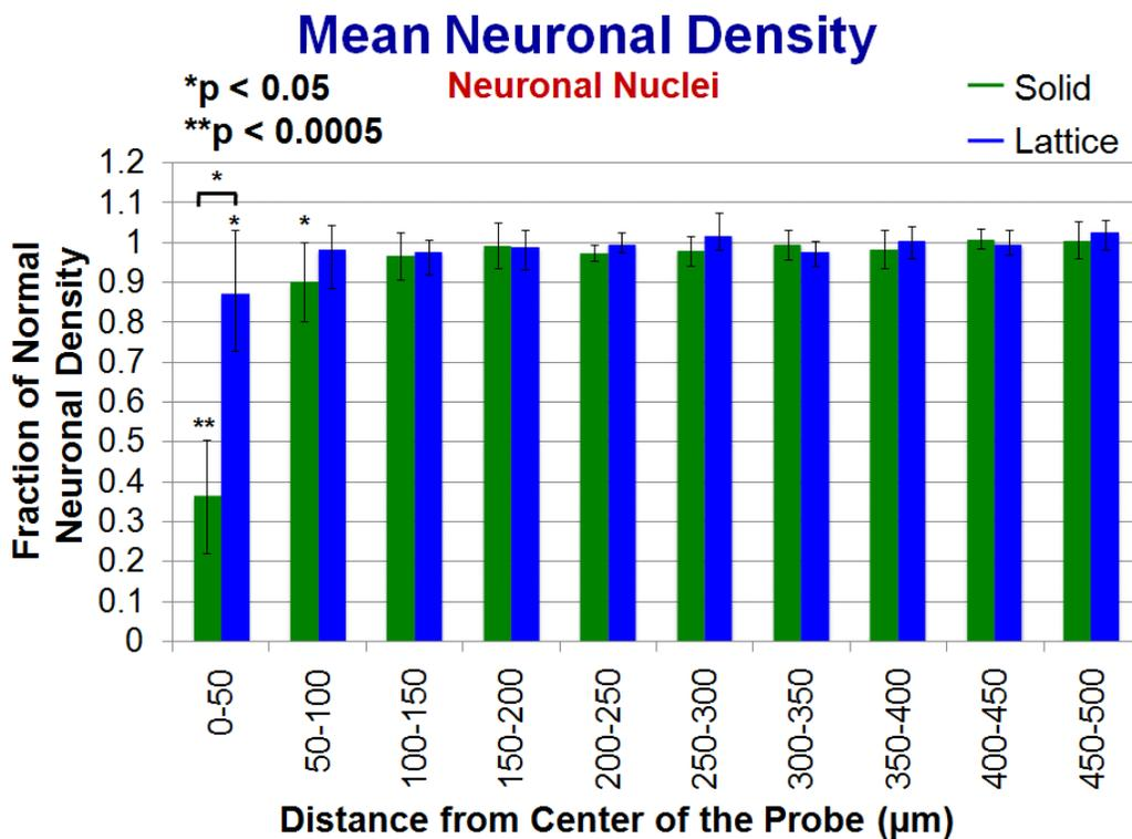
Fig. 2.18: Horizontal section with overlay of the 50µm bins (top) and quantitative data of the NeuN biomarker distribution (bottom) [84]. The first bin shows a statistically significant difference ( $p < 0.05$ ) in NeuN density between the solid and lattice architecture with a substantial increase in the chronic neuronal survival for the lattice probe (87%) over the solid device (36%) as a percentage of background (400-500µm bins) NeuN density.
