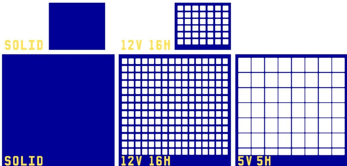
Fig. 2.4: Layout of stand-alone platforms to study effects of occluded cortical surface area. The smaller version has a footprint of  $600\mu\text{m}$  by  $500\mu\text{m}$  and the larger one is  $1200\mu\text{m}$  by  $1200\mu\text{m}$ . The widths of the vertical and horizontal supports are indicated in the image for each design.
