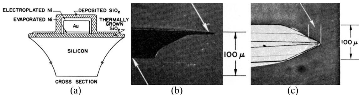
Fig. 1.1: Single electrode microprobe (a) cross sectional drawing and (b) side view and (c) top view photomicrographs, cropped from [3].
