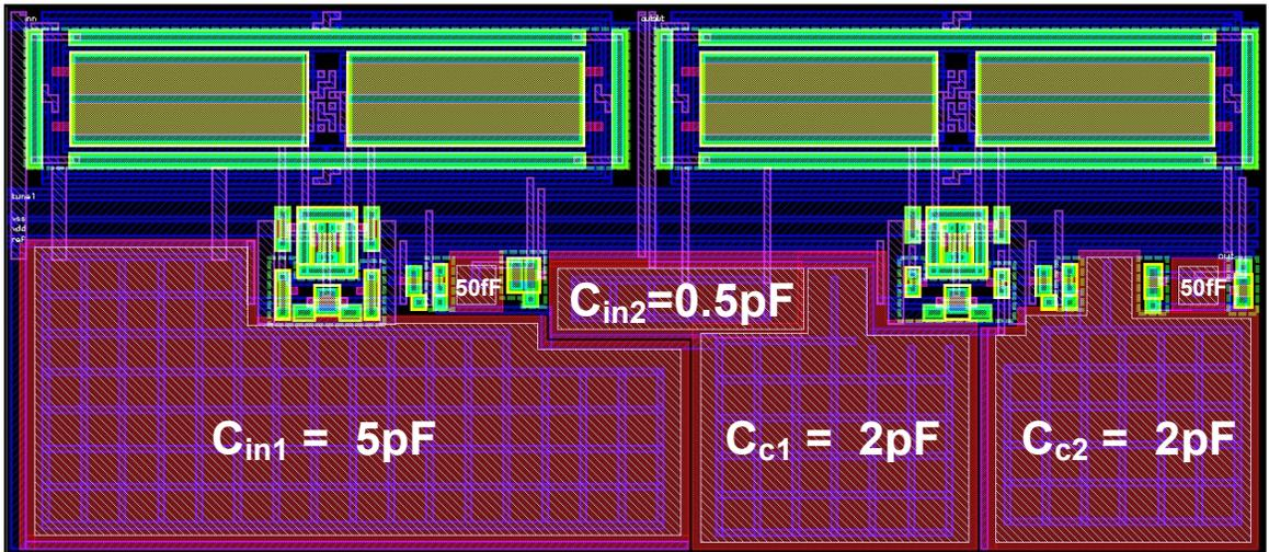
Fig. 4.4: Dual-stage 60dB amplifier layout in  $0.0255\text{mm}^2$  ( $243.45\mu\text{m} \times 104.85\mu\text{m}$ ) with a simulated power dissipation of  $51.51\mu\text{W}$ , excluding the shared bias.
