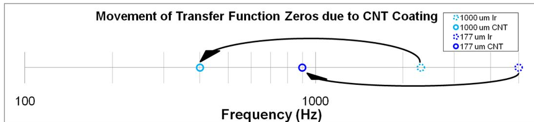
Fig. 3.10: Graph showing movement of the zeros in the modeled transfer function.
