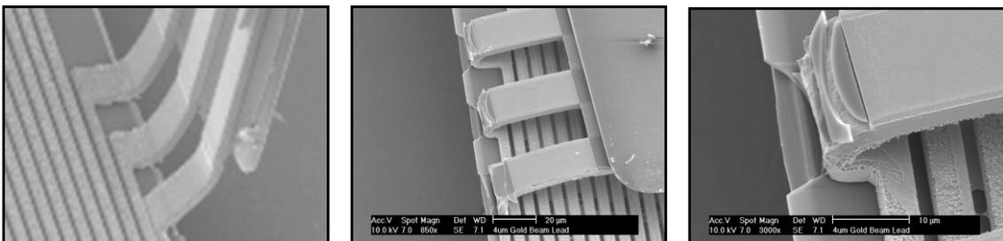
Fig. 5.28: SEMs of forward bends showing inherent challenges.
