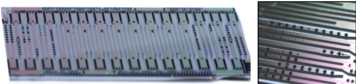
Fig. 3.15: Photographs of CNT growth (30sec) on non-released probes.
