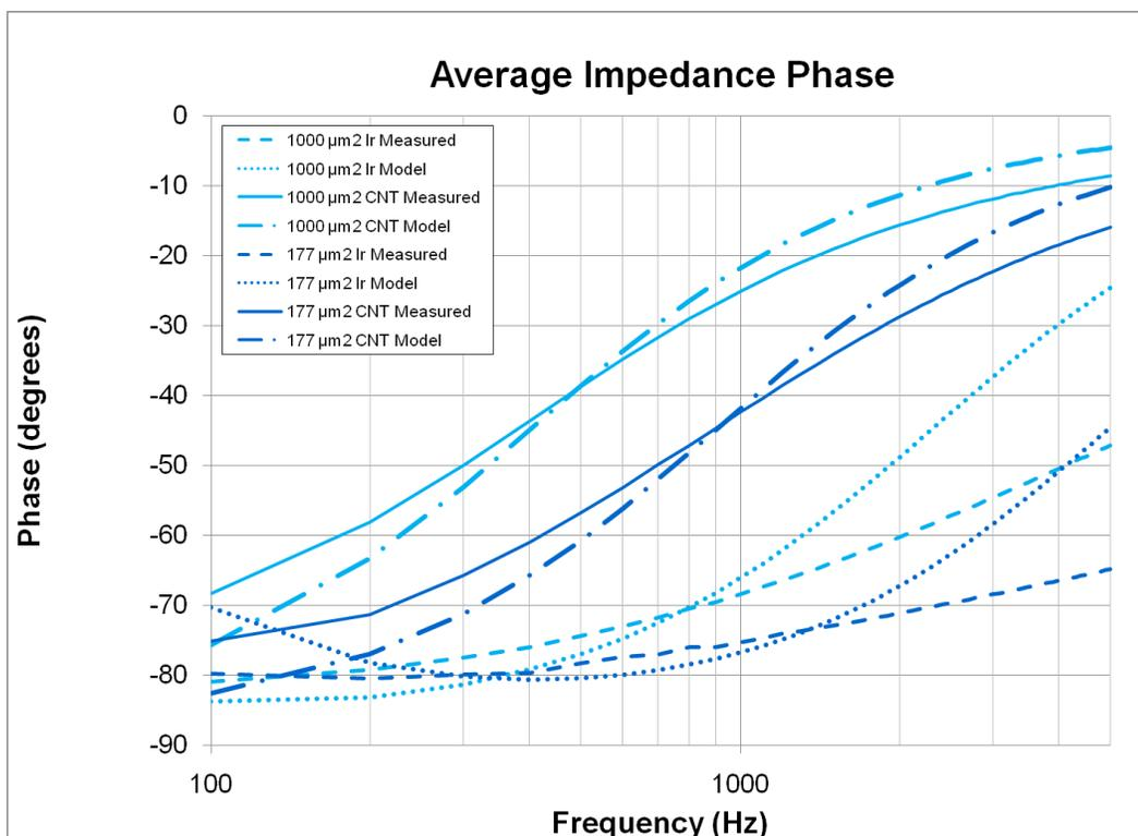
Fig. 3.7: Average of measured impedances of good iridium sites (dashed) and CNT dip-coated sites (solid), with areas of  $177\mu\text{m}^2$  (dark blue) and  $1000\mu\text{m}^2$  (light blue). Parameter-fit with Randles model is also shown, see Section 3.3.3.
